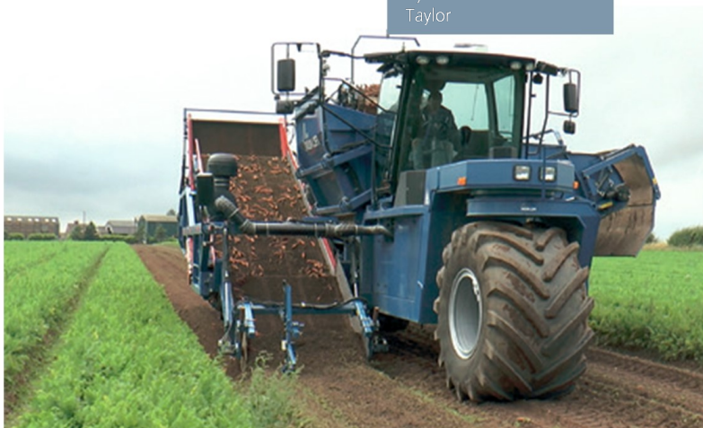
Investment in the new ASA-self-propelled carrot harvester, designed and developed by ASA-lift and Nick Taylor
